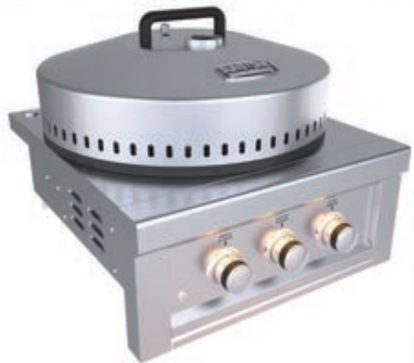
SUNSTONE® 24" POWER CIRQUE™ BURNER Item No: SUN24PCB Product Size: 24"W x 26-1/2"D x 18-1/2"H FireBox Size: 22-1/4"W x 22-1/4"D x 9"H Cut-out: 22-3/4"W x 22-1/2"D x 10"H
