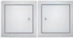
12" X 12" SINGLE UTILITY ACCESS DOOR Item No: BA-SD12 Product Size: 12"W x 12"H x 3"D Cut-out: 10-1/4"W x 10-1/4"H
