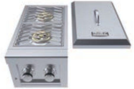
RUBY SERIES 13" SLIDE IN VERSA DOUBLE BURNER Item No: SUN13VDB-LP/NG Product Size: 13"W x 23-1/2"D x 12-1/2"H Cut-out: 12"W x 20-1/4"D x 9"H Up To 30,000 BTU's • LED Light on Control Panel
