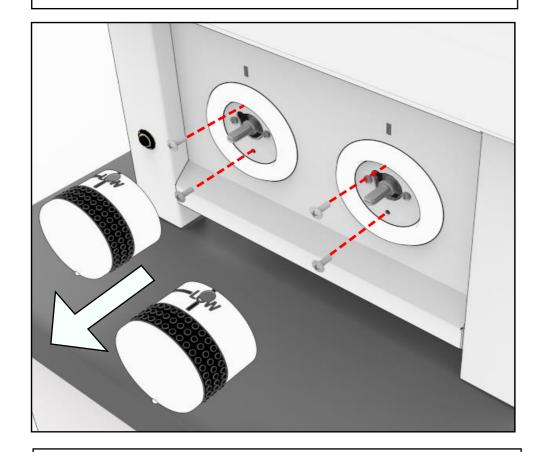
7. USE SCREW DRIVER TO REMOVE THE TWO PANEL SCREWS IN PORT HOLES.
