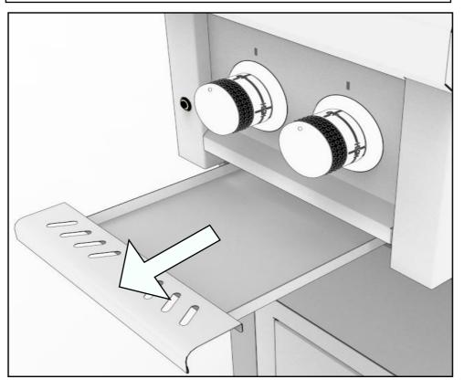
3. TURN KNOBS COUTNER-CLOCKWISE TO REVEAL HOLE, USE ALLAN WRENCH TO REMOVE KNOBS. (ALLAN WRENCH IS INCLUDED IN YOUR MANUAL BAG)
