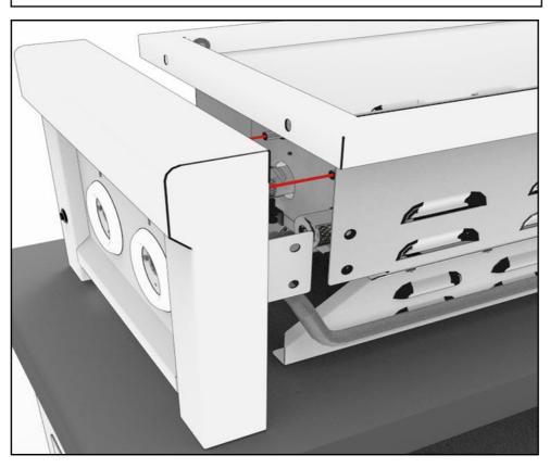
6. REMOVE THE COVER, COOKING GRID AND FLAVORIZER RACK INSIDE GRILL
