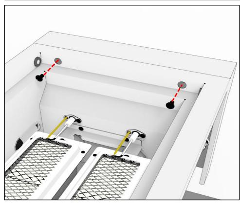
6. REMOVE MANIFOLD PIPE BRACKET LOCATED IN BACK OF GRILL FOR LP TO NG CONVERSION ONLY!
