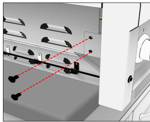
8. SLIDE CONTROL PANELFORWARD, LEAVING VALVES ATTACHED TO MANIFOLD.
