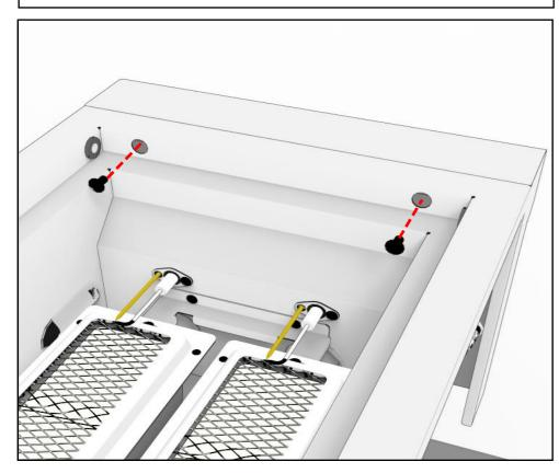
5. REMOVE BOTH LEFT/RIGHT SIDES TWO SCREWS.
