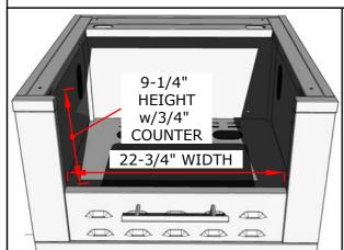
Removing top panel allows a product insert dimension of 22-3/4" Width x 8-1/2" Height x Max 24-1/2" Depth Add 1 Inch Height Counter to provide a Cut-Out height of 9-1/2"
