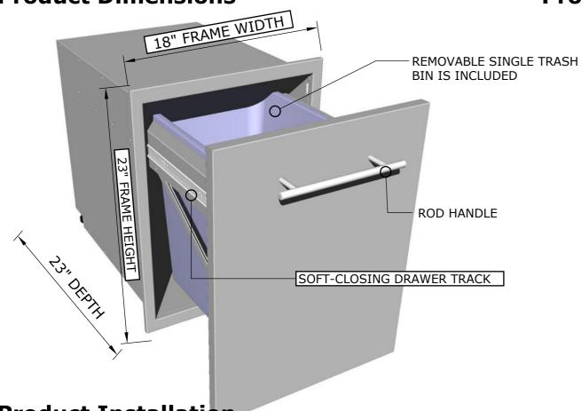
COMBINE MULTIPLE COMPONENTS TOGETHER INTO UNLIMITED COMBINATIONS A 1/16" RAISED FRAME VISIBLE EDGE ENABLING OU TO PLACE TWO OR MORE COMPONETS SIDE BY SIDE OR ONTOP OF ONE ANOTHER CREATING ONE SINGLE LARGER FUNCTIONING COMPONET OF YOUR OWN CHOOSING DE-TRD18 DE-DPCF23
