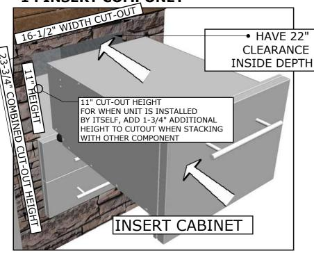
**IMPORTANT!! -** ROD HANDLES ARE MOUNTED TO INSIDE OF PANEL,
