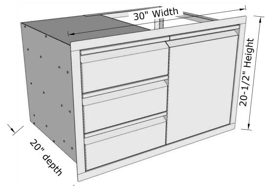
MOUNT TO INTERIOR ISLAND CUT-OUT EDGE USING SCREW CONSISTENT WITH YOUR INSTALLATION TYPE. CONCRETE, MASONRY, WOOD, METAL ALL USE DIFFEREANT SCREW TYPES (HARDWARE NOT
