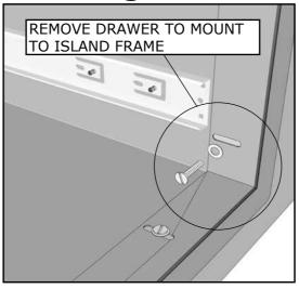
HAVE COMPONENT ON SITE BEFORE MAKING ISLAND CUTS, CONFIRM ALL DIMENSIONS BEFORE CUTTING INTO ISLAND WALL
